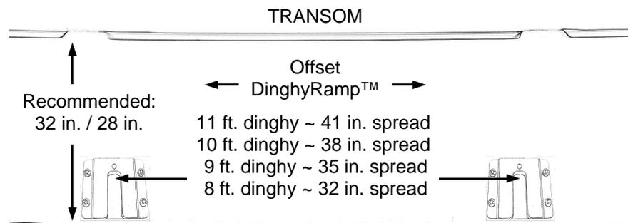
**Step 2** - Place mounting brackets (#QUICKKIT) on the edge of the swim platform. Adjust mounts so they are parallel and facing aft.
